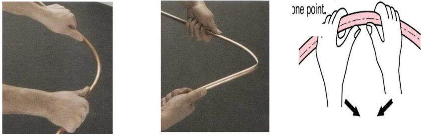
Manual bending of pipe
