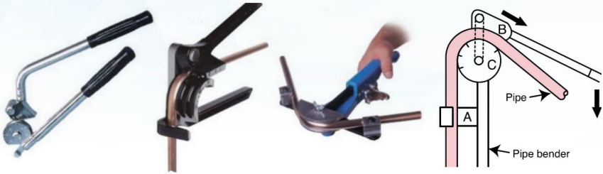
Bending by pipe bender
